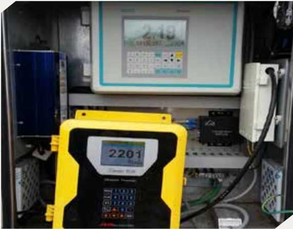
Foreign Ultrasonic Flowmeter(Top) and Jain Technology Ultrasonic Flowmeter(Bottom) (K-Water Profit Sharing Task 2014)
